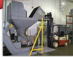
Operators feed 3/4-cubic-yard carts of chips and turnings into the PRAB automated chip processing system's vertical axis crusher. The crusher reduces the metal scrap six times in volume to produce flowable chips.
