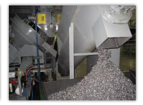
A screw conveyor dispenses the dry chips into a cart for easy transport. The PRAB system effectively reduces the volume of metal waste 600 percent and recovers 99.6 percent of oils, or about 300 gallons (1,135 liters) per day.
