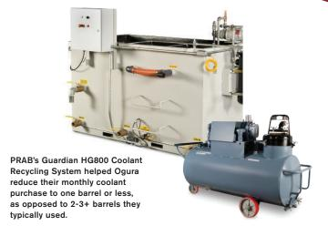
After the incorporation of the HG-800 coolant recycling system into Ogura's operations, make up coolant usage went from two to three barrels of coolant per month to just one barrel or less per month. In the first 12 months after installing the PRAB Guardian recycling system Ogura did not need to haul away any coolant.
