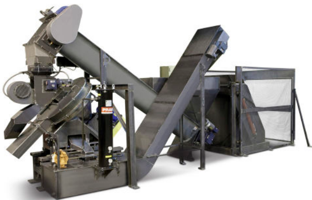
Wringer can be integrated with other PRAB equipment for a complete chip processing system.
