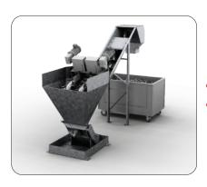
The PRAB Bundle Breaker is installed in a conveyor's in-feed hopper. The unit may be added to an existing conveyor or incorporated into a new PRAB metal scrap processing system.
