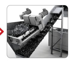
When bushy wads of metal scrap are deposited into the hopper, the Bundle Breaker's dual rotating cylinders agitate the material, tearing apart stringy wads of turnings.
