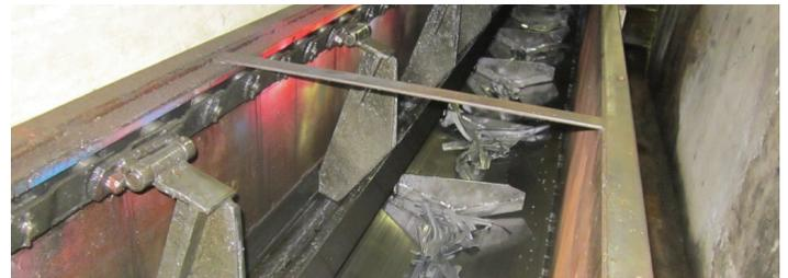
The PRAB ScrapVeyor™, shown here, includes a lube system that automatically greases bearings. This feature decreases routine maintenance.
