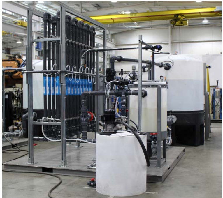
Pictured Above: PRAB Tubular Ultrafiltration system used to treat oily wastewater consisting mostly of used die lube and mop bucket/floor scrubber water. This system was custom designed with twenty-two Porex Tubular Membranes (1" in diameter by 6' long) that were vertically mounted to minimize floor space.
