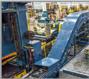
A heavy duty steel belt conveyor collects stamping scrap when no pit is available. The conveyor elevates and discharges into large scrap containers. Available on wheels for even faster die changes.
