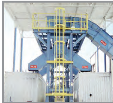
A load-out system provides even distribution into containers for high volume applications. Systems are engineered for new spaces or integrated into existing infrastructure.
