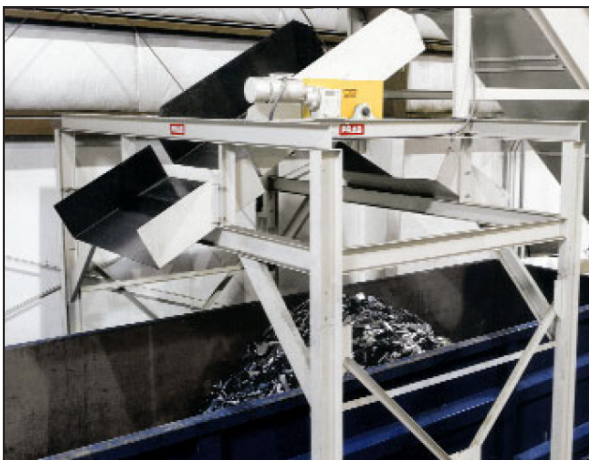
(2) A tipping chute (automatic or manual) for a single full size trailer or two smaller containers, side-by-side
