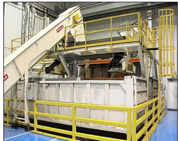
(3) An automatic shuttle conveyor chute system for even loading of dual full size trailers
