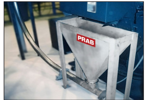
Typical chips and coolant inlet receiver hopper from CNC machine
