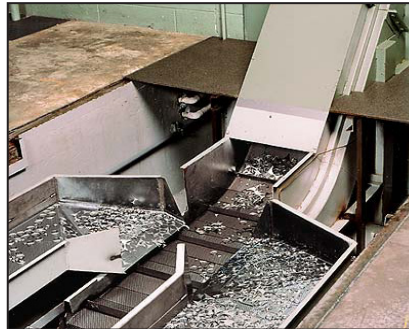
Oscillators can be used with steel belt conveyors for complete systems
