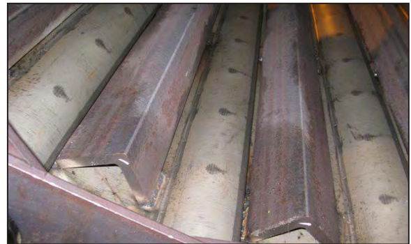
Optional inverted flights for high temperature applications
