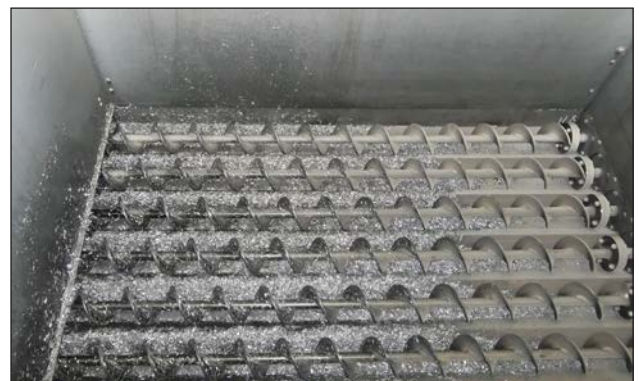
Live bottom hopper includes multiple 6" augers
