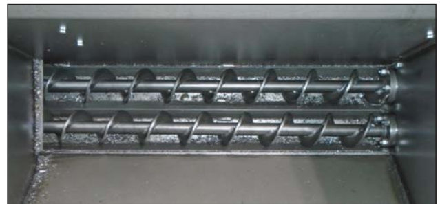
1/2 Yard infeed hopper includes two 3" augers
