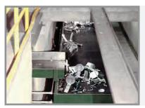
Scrap aluminum from die cast trim presses drop onto oscillating conveyors that feed onto dual under-floor centralized collection oscillators.
