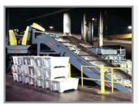
Oscillating conveyor deposits scrap into a large 6" pitch steel belt conveyor for elevation.
