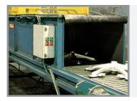
A casting cooler uses single or multiple cooling zones for cooling hot die castings.
