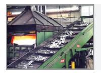
Furnace feeders allow for meter feeding abrasive die casting metal scrap directly to a melting furnace.
