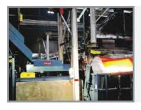
Scrap discharges onto a swivel chute that feeds furnace feeders equipped with replaceable stainless steel sections that extend into the melt area of the furnace.
