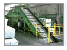
Steel belt conveyor elevates dry and wet scrap, chips and parts.
