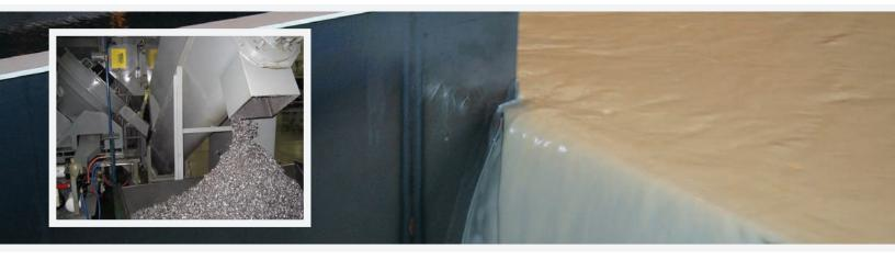
Previously, the company's scrap removal process involved collecting material saturated with cutting fluid in a self-dumping hopper off of its gantry mill and discharge conveyor. A forklift would then pick up the full hopper and take it to a larger hopper or lugger box outside to be hauled away by the recycler.
