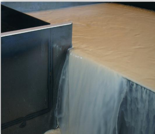
*PRAB's Guardian Coolant Recycling System utilizes a continuous overflow process to prevent rancidity.*
