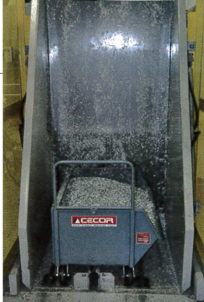
Chips are temporarily stored in a metal tote before entering a central processing system.
