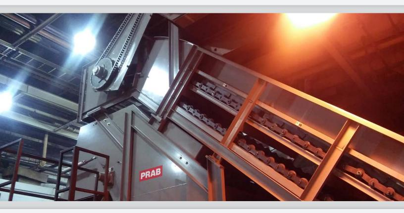
A die casting plant that manufactures all aspects of automotive transmissions, from die cast parts through final assembly, needed to reduce downtime associated with re-melting scrap material created during the casting process. The plant's scrap output was as much as 20,000 lbs./hour, and the scrap sizes ranged from 1/4" pieces to 70-lb. transmission housings.
