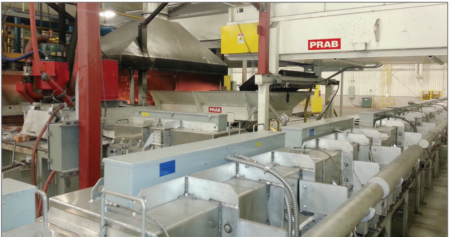
PRAB Z Style Steel Belt Conveyor deposits scrap, without carry over, onto a furnace feeder. The furnace feeder evenly deposits scrap into the furnace.
