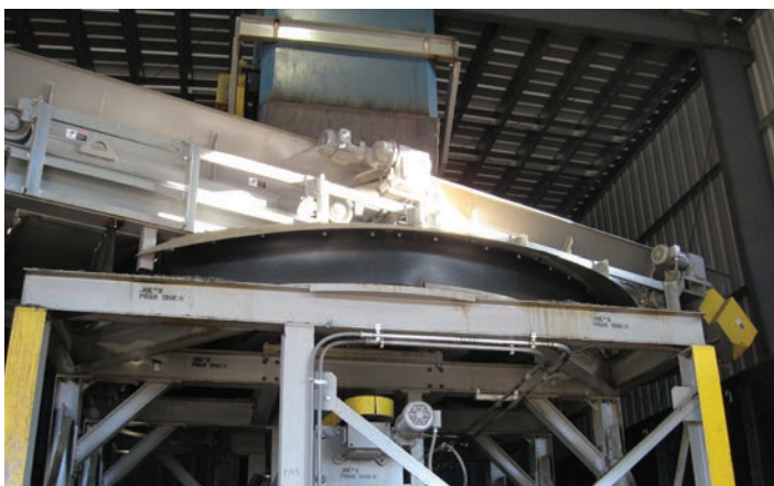
Orbital Shuttle rotates a traversing steel belt conveyor between two parallel containers. Programmable controls automate the entire filling process.
