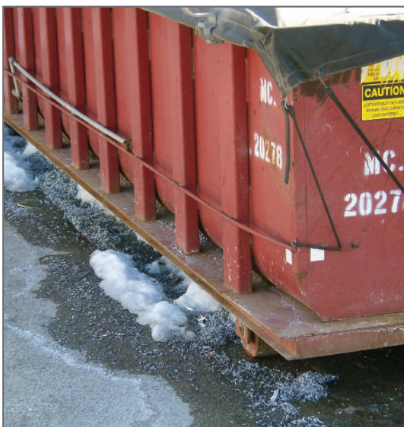
Martin-Baker's original waste management process included machinists dumping hoppers of loose aluminum chips into roll-off hoppers in the plant's parking lot.
