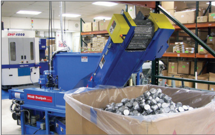
PRAB's Dualpak™ briquetter reduces the volume of aluminum chips, recovers valuable coolant and improves machinist productivity and safety.
