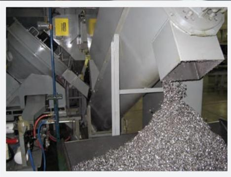
Previously, the company's scrap removal process involved collecting material saturated with cutting fluid in a self-dumping hopper off of its gantry mill and discharge conveyor. A forklift would then pick up the full hopper and take it to a larger hopper or lugger box outside to be hauled away by the recycler.
